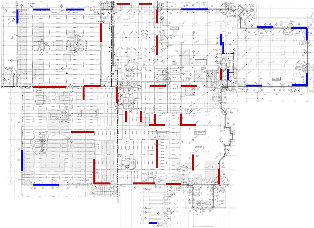
Figure 12: Braced Frames Location
